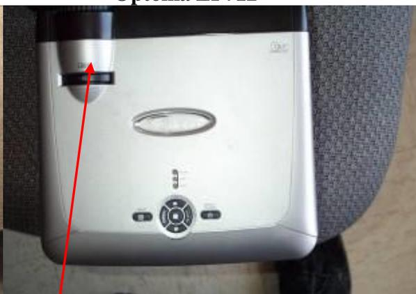
*Zoom and focus adjustments are made through the lens*
